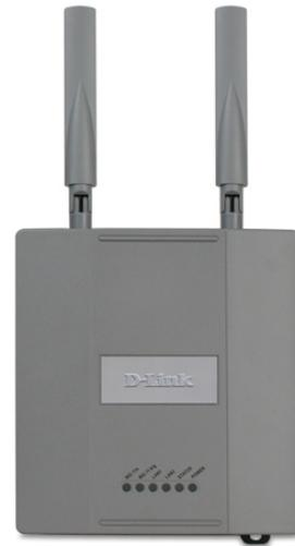
The DWL-8200AP delivers excellent wireless performance with maximum flexibility, enabling two parallel networks to be set up for organisations that want to ensure optimum accessibility and scalability. With its onboard SuperG function engaged, it is possible to achieve even greater performance of up to 108Mbps in 802.11g mode.
