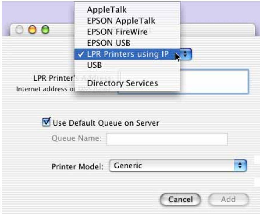
4. In the text box called **LPR Printer's Address**, type in the IP address of the print server. Deselect “**Use Default Queue on Server**” and specify the port name of the printer port on the print server.
