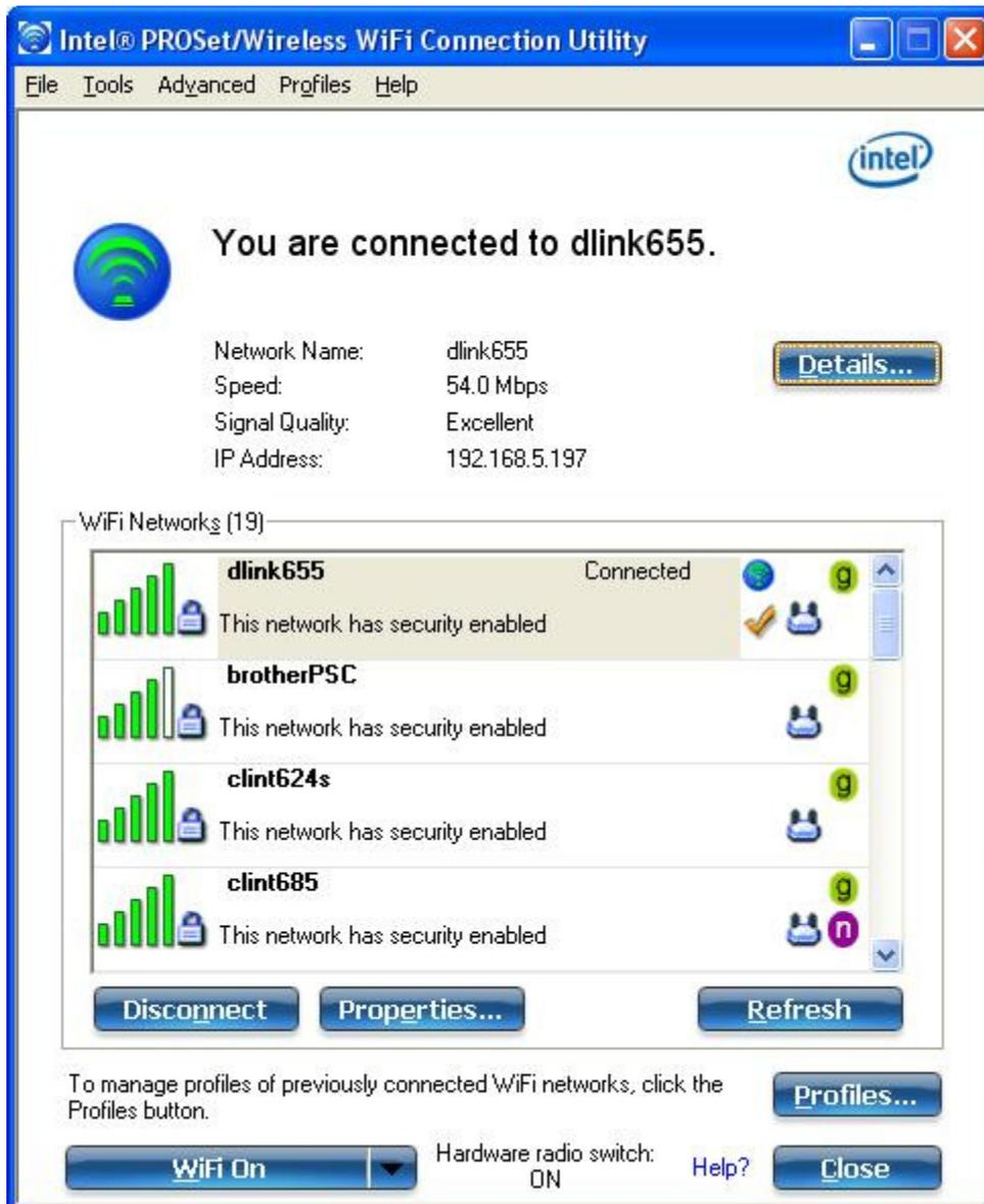
18. To check whether both units are broadcasting the same **SSID**, select your networks **SSID** in the list of available networks and click the **PROPERTIES** button.
