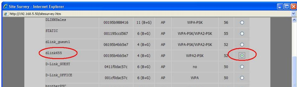
14. Enter the WEP or WPA-PSK (passphrase) in the field required to complete the setup. **The Site Survey scan will auto-fill the rest of the fields such as the type of security the primary router / AP is using.**
