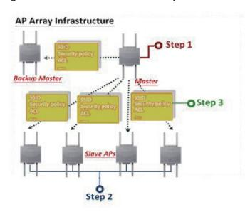
Up to eight stand-alone APs can be managed in an array. Members in the same AP Array group must be on the same subnet of the same model, and each AP is assigned with a unique IP address.
