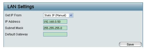
**IP Address:** The default IP address is **192.168.0.50**. Assign a static IP address that is within the IP address range of your network.
