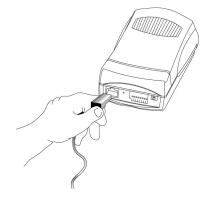
• Attach the External Power Supply Attach the external power supply to the DC power input connector located on the DCS-1000's rear panel and is labeled DC 5V and connect it to your local power supply.
