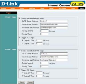
These fields control Input Trigger 1 and Trigger 2. Each Input Trigger can trigger either or both Output triggers.
