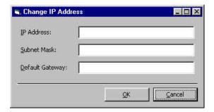
Enter the new IP Address, the Subnet Mask and the Default gateway into the respective fields and click OK. IPView will automatically change the IP Address.
