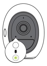
Once at the camera is synced successfully, the LED on the camera will illuminate green to indicate it's currently connected.
