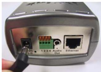
When you have a proper connection, the **LED** (Light Emitting Diode) on the front of the camera will turn from red to green. The light may blink on and off and your computer may show an intermittent loss of connectivity if you have it directly connected to the camera. This is normal until you have configured your camera.
