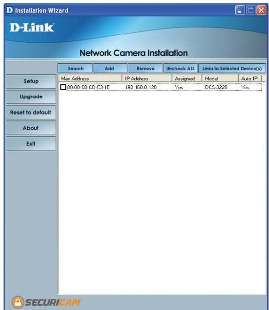
\*A DHCP server is a device that supplies IP Addresses to its clients that are on the same network.
