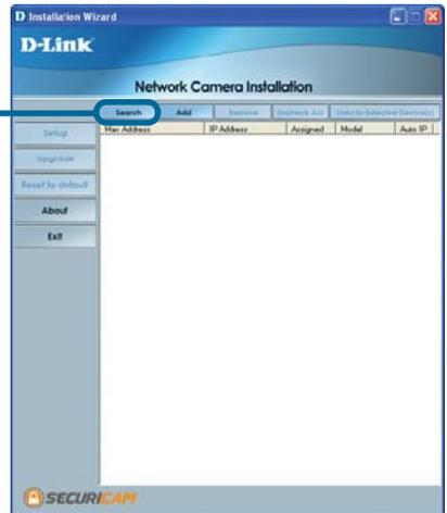
Once the camera appears, select the camera by placing a **Checkmark** in the box.
