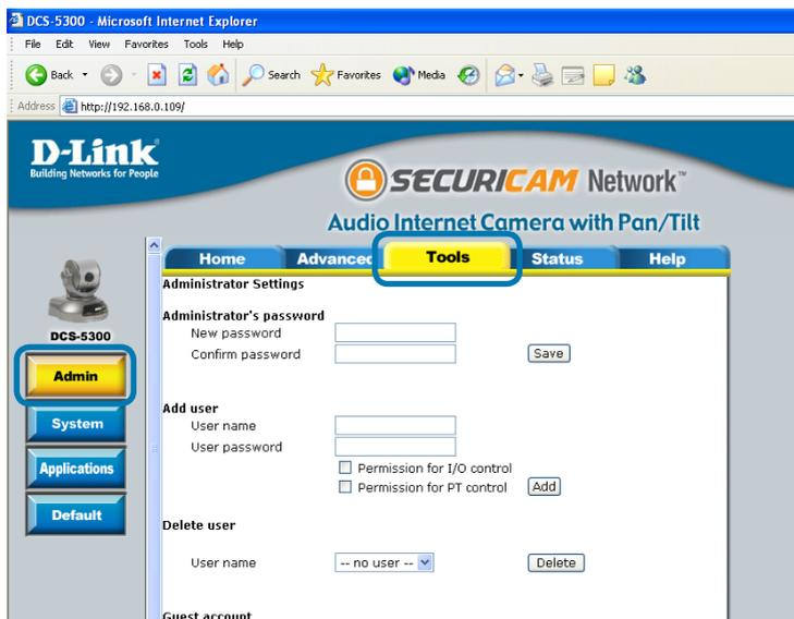
The **DCS-5300** is manufactured without any passwords by default. This allows the ability to access the **DCS-5300** (including the Configuration) by anyone as long as the IP address is known. It is recommended that you enter a password to restrict others from accessing your camera.
