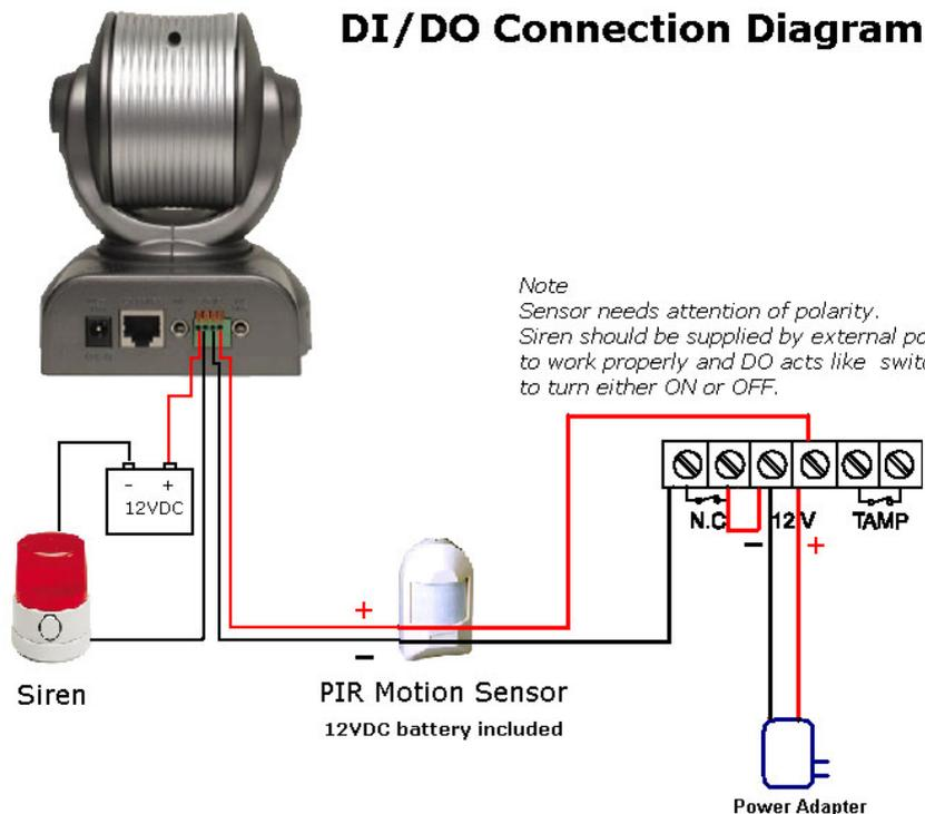
The above diagram shows a typical wiring configuration for a normally closed PIR motion sensor. Please refer to your specific motion sensor for the power supply connection to the device since this will be critical to the success of your installation. Note that the positive from the PIR is connected to the D+ of the I/O port of the camera and the negative from the PIR is connected to the D- of the camera I/O port.
