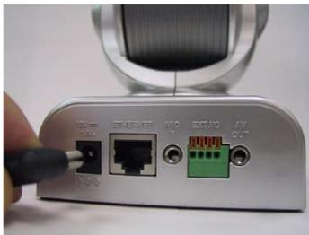
When you have a proper connection, the LED will turn from **red** to **green**. If you are directly connected to the camera via a crossover cable, the light may cycle on and off and your computer may show an intermittent loss of connectivity. This is normal until you have configured your Internet Camera.
