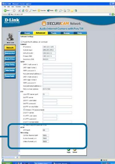
These are the port settings for your camera. If necessary, these ports can be changed if they are already in use by other devices (e.g. in a multiple camera environment).
