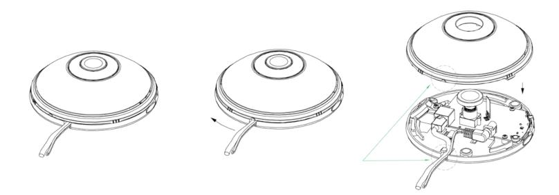
You can access the inside of the DCS-6010L by rotating the camera cover counter-clockwise, then lifting it off of the camera.
