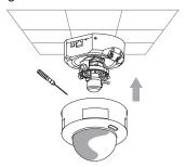
Place the ring enclosure over the dome enclosure. Once placed, gently turn the ring enclosure clockwise until it locks and is securely attached to the dome enclosure.
