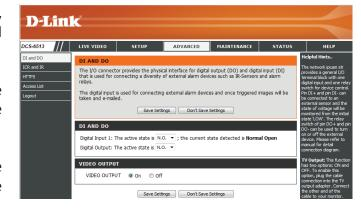
Video Output: Enable/ disable the BNC terminal TV output signal.
