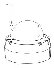
**Disassemble the Camera**Open the camera enclosure by loosen the 4 screws. Lift the dome off the base of the camera.
