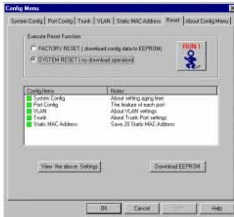
Figure 5.11 Screen shot of the system reset of the Switch Configuration Software
