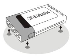
Figure 2-2. Attaching the Rubber Feet
