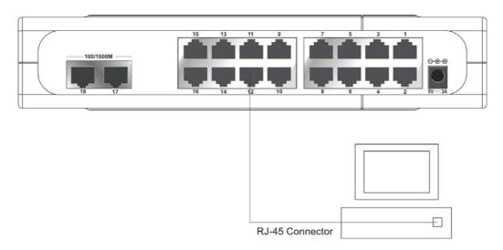
Figure 3-1. Switch connected to an end node
