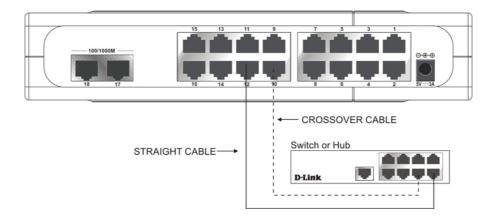
Figure 3-2. Switch connected to a port on a hub or switch using either a straight or crossover cable—any normal cable is fine
