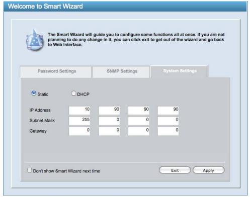
Figure 27 - Configure System IP address in Smart Wizard
