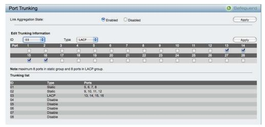
Figure 46 - Configuration > Link Aggregation > Port Trunking
