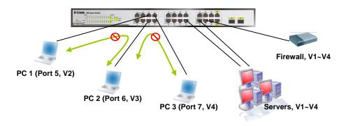
Figure 49 - Configuration > 802.1Q VLAN > Asymmetric VLAN Example
