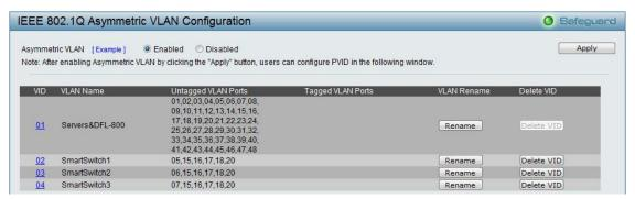
Figure 41 - Configuration > 802.1Q VLAN > Asymmetric VLAN - Create VLANs
