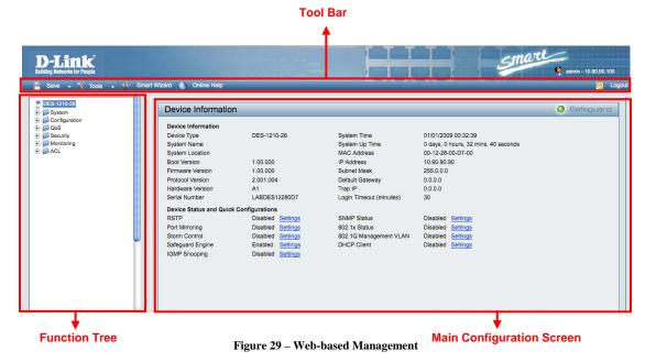
Above is the Web-based Management screen. The three main areas are the **Tool Bar** on top, the **Function Tree**, and the **Main Configuration Screen**.
