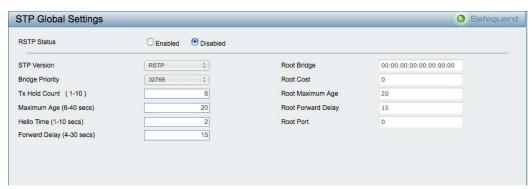
Figure 53 – Configuration > Spanning Tree > STP Global Settings
