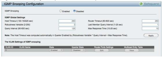
Figure 54 - Configuration > IGMP Snooping Configuration
