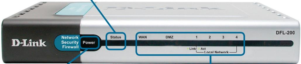
**POWER LED** – a solid light indicates a proper connection to the power supply.
