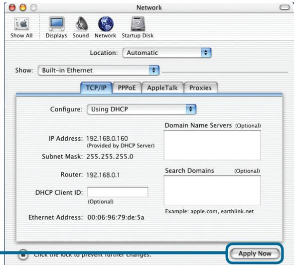
The IP address information, the Subnet Mask, the DFL-200 IP address and the Ethernet adapter address will appear
