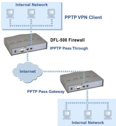
Configure the PPTP VPN client to connect to the destination PPTP VPN gateway as if the client computer is connected directly to the Internet.
