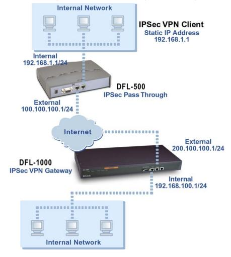
IPSec client connecting to a VPN on the Internet using VPN pass through
