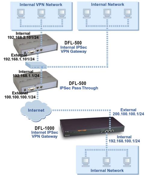
Use the following procedures to configure the internal IPSec VPN gateway, the Internet IPSec VPN gateway, and the DFL that will be passed through.
