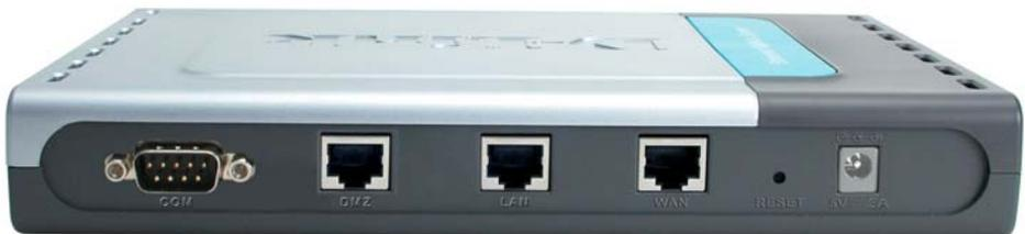
**COM Port:** Serial access to the firewall software, 9600, 8bit, None Parity, 1Stop bit.
