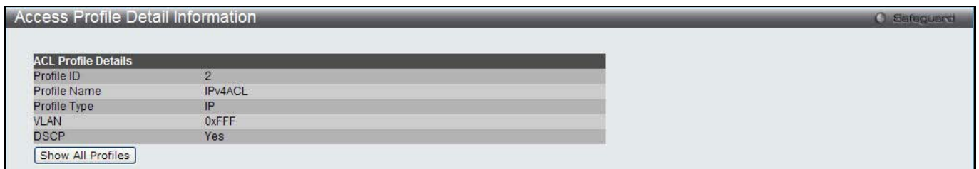
Figure 7-9 Access Profile Detail Information window (IPv4 ACL)
