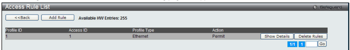
Figure 7-5 Access Rule List window (Ethernet ACL)
