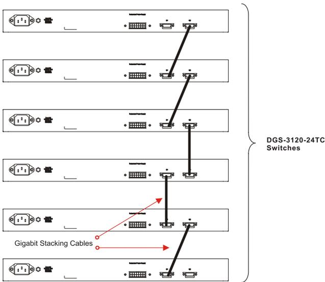
Figure 2-32 Switches stacked in a Duplex Chain
