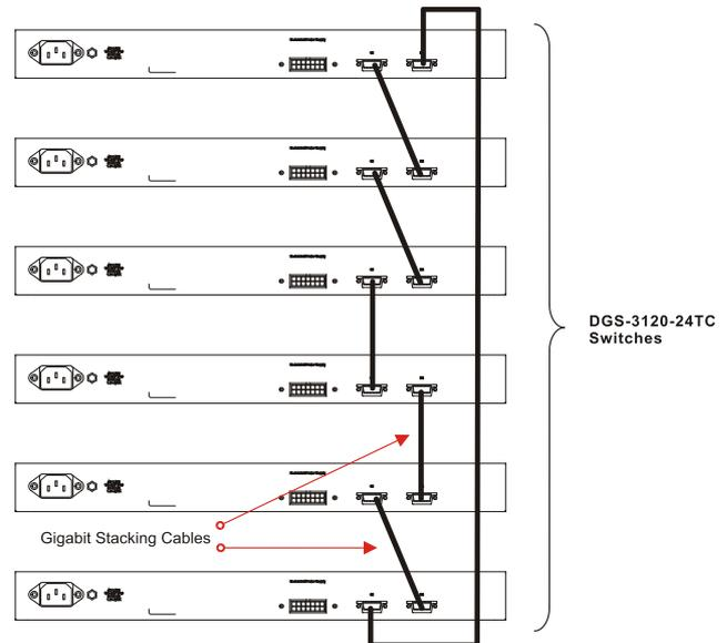
Figure 2-33 Switches stacked in a Duplex Ring
