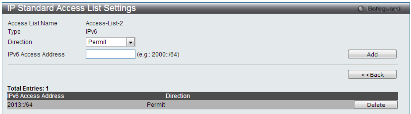
Figure 6-187 IP Standard Access List Settings - View Detail (IPv6) window
