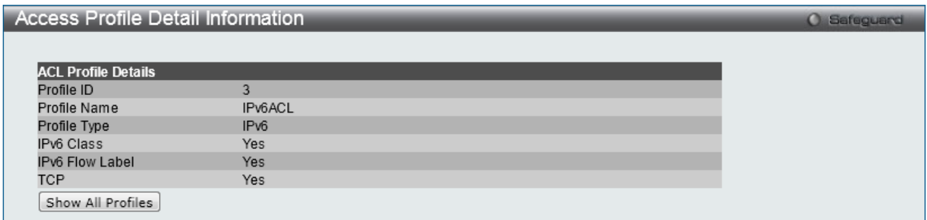
Figure 8-14 Access Profile Detail Information window (IPv6 ACL)
