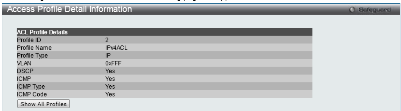
Figure 8-9 Access Profile Detail Information window (IPv4 ACL)
