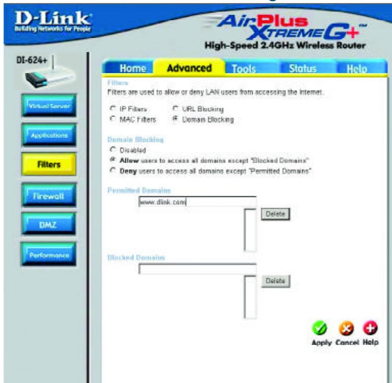
Domain Blocking is used to allow or deny LAN (Local Area Network) computers from accessing specific domains on the Internet. Domain blocking will deny all requests to a specific domain such as http and ftp. It can also allow computers to access specific sites and deny all other sites.
