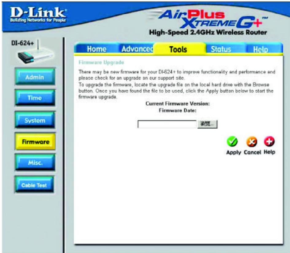
You can upgrade the firmware of the Router here. Make sure the firmware you want to use is on the local hard drive of the computer. Click on **Browse** to browse the local hard drive and locate the firmware to be used for the update. Please check the D-Link support site for firmware updates at <http://support.dlink.com> or global websites. You can download firmware upgrades to your hard drive from the D-Link support site.
