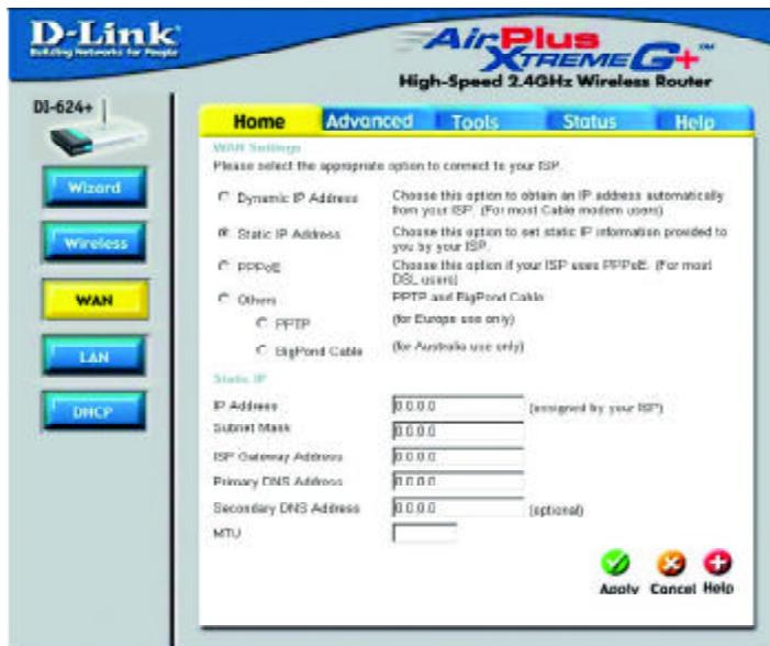
**Static IP Address-** Choose Static IP Address if all WAN IP information is provided to you by your ISP. You will need to enter in the IP address, subnet mask, gateway address, and DNS address(es) provided to you by your ISP. Each IP address entered in the fields must be in the appropriate IP form, which are four octets separated by a dot (x.x.x.x). The Router will not accept the IP address if it is not in this format.
