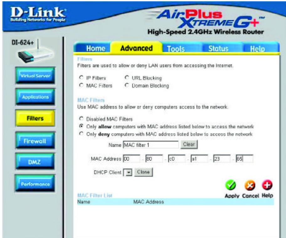
Use MAC (Media Access Control) Filters to allow or deny LAN (Local Area Network) computers by their MAC addresses from accessing the Network. You can either manually add a MAC address or select the MAC address from the list of clients that are currently connected to the Broadband Router.
