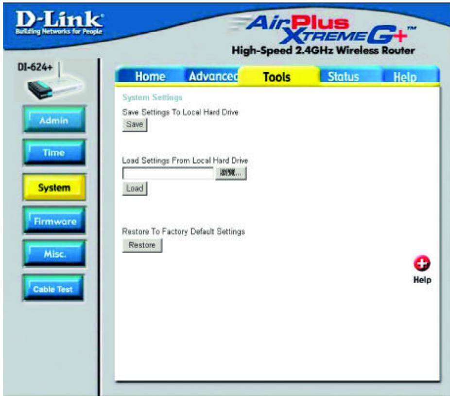
The current system settings can be saved as a file onto the local hard drive. The saved file or any other saved setting file can be loaded back on the Broadband Router. To reload a system settings file, click on **Browse** to browse the local hard drive and locate the system file to be used. You may also reset the Broadband Router back to factory settings by clicking on **Restore**.
