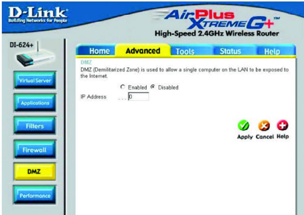
If you have a client PC that cannot run Internet applications properly from behind the DI-624+, then you can set the client up for unrestricted Internet access. It allows a computer to be exposed to the Internet. This feature is useful for gaming purposes. Enter the IP address of the internal computer that will be the DMZ host. Adding a client to the DMZ (Demilitarized Zone) may expose your local network to a variety of security risks, so only use this option as a last resort.
