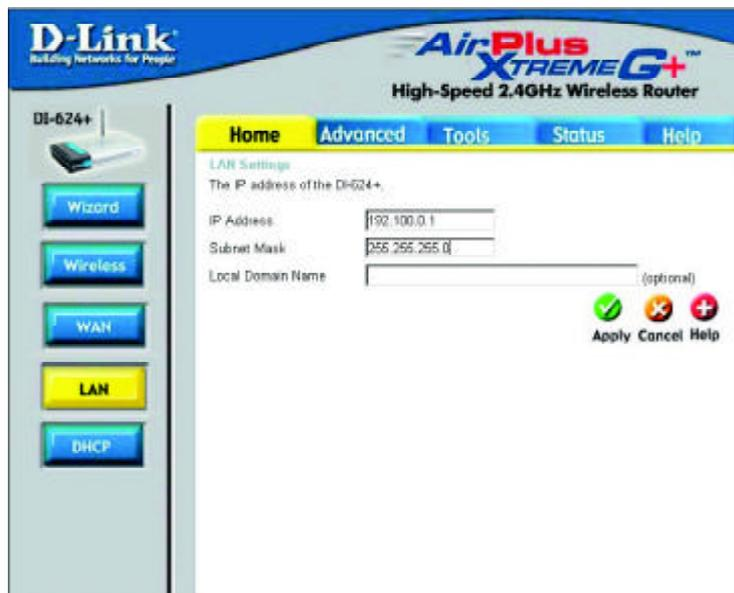
LAN is short for Local Area Network. This is considered your internal network. These are the IP settings of the LAN interface for the DI-624+. These settings may be referred to as Private settings. You may change the LAN IP address if needed. The LAN IP address is private to your internal network and cannot be seen on the Internet.
