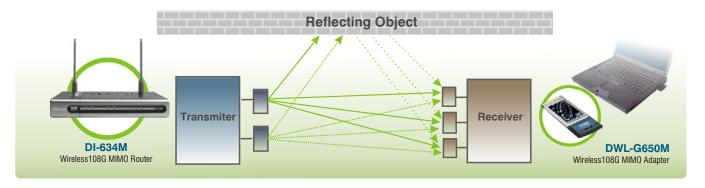
Wireless 108G MIMO (Multiple Input, Multiple Output)
