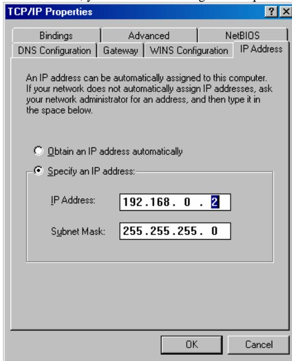
The Gateway on EACH PC has to be the IP address of DI-701 (192.168.0.1 in this example) because it is the “door” way to get out to Internet through ADSL.
