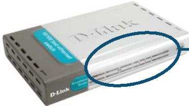
**LAN Port LEDs.** Each of the LAN ports on the back of the DI-704P have a corresponding LED light on the front panel of the unit. When a proper connection has been made to a computer that is ON, the LED on the front panel should illuminate.
