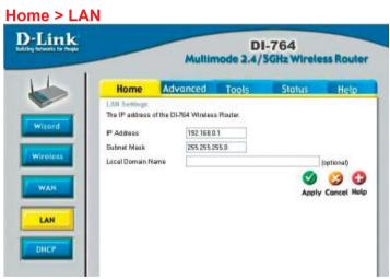
LAN is short for Local Area Network. This is considered your internal network. These are the IP settings of the LAN interface for the DI-764. These settings may be referred to as Private settings. You may change the LAN IP address if needed. The LAN IP address is private to your internal network and cannot be seen on the Internet.
