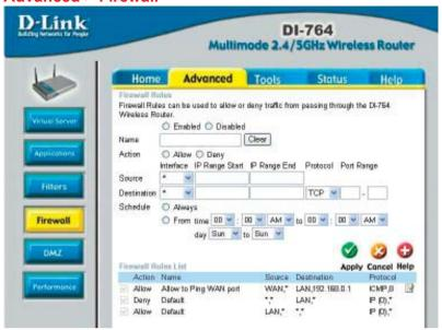
**Firewall Rules** is an advanced feature used to deny or allow traffic from passing through the DI-764. It works in the same way as IP Filters with additional settings. You can create more detailed access rules for the DI-764. When virtual services are created and enabled, it will also display in Firewall Rules. Firewall Rules contains all network firewall rules pertaining to IP (Internet Protocol).
