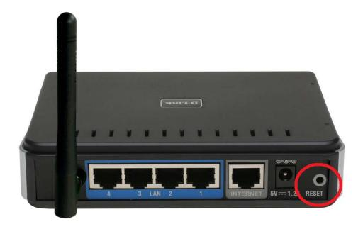
2. Insert a paperclip into the reset pin hole and hold in for 10 seconds. While holding in the reset button, refer to the Status LED, when it starts to blink rapidly, release the paperclip holding in the reset button.
