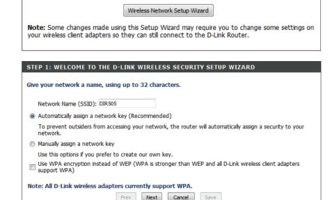
This wizard is designed to assist you in your wireless network setup. It will guide you through step-by-step instructions on how to set up your wireless network and how to make it secure.
