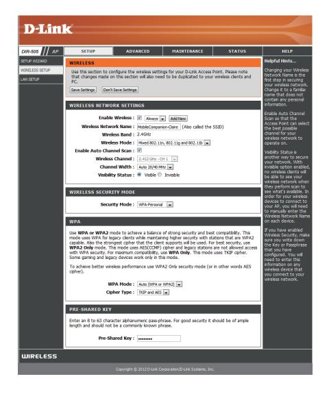
Wireless Indicates the channel setting for the DIR-505. The Channel Channel: can be changed to fit the channel setting for an existing wireless network or to customize the wireless network. If you enable Auto Channel Scan, this option will be grayed out.
