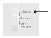
If this is your first time configuring the DIR-505, open your web browser and type **http://dlinkrouter** in the address bar. You will automatically be directed to the **Wizard Setup Screen**. For more information, refer to "Initial Setup Wizard (Router/AP Mode)" on page 15.
