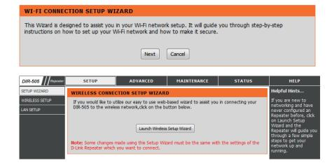
Select **WPS** as the configuration method only if your wireless device supports Wi-Fi Protected Setup (WPS). For **Manual** setup, skip to the next page.
