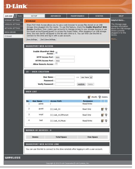
**Number of** This section shows you information about the USB storage **Devices:** device plugged into the router.
