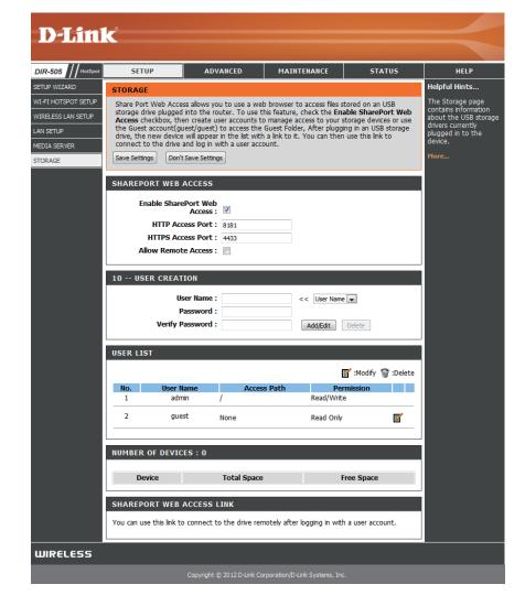
**Number of** This section shows you information about the USB storage **Devices:** device plugged into the router.
