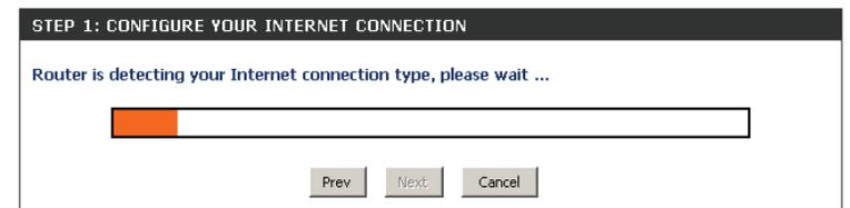
If the router does not detect a valid Ethernet connection from the Internet port, this screen will appear. Connect your broadband modem to the Internet port and then click **Try Again**.
