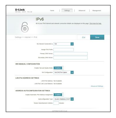
LAN IPv6 Link- Displays the router's LAN link-local address.
