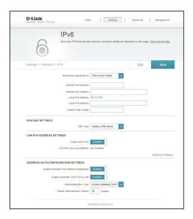
LAN IPv6 Link- Displays the router's LAN link-local address. **Local Address: Enable** Enable or disable the Automatic IPv6 Address Assignment feature. **Automatic IPv6 Address Assignment: Enable** Enable or disable automatic DHCP-PD services. **Automatic DHCP-PD** in LAN: Auto Select SLAAC + RDNSS, SLAAC + Stateless DHCP, or Stateful Configuration (DHCPv6). Type: Router Enter the IPv6 address lifetime (in minutes). **Advertisement** Lifetime: Click **Save** when you are done.
