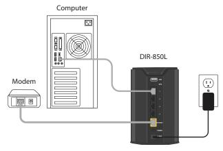
7. If you are connecting to a broadband service that uses a dynamic connection (not PPPoE), you may be online already. Try opening a web browser and enter a web site. A solid light indicates a connection on the Internet port and the router can connect to the Internet. If the LED is orange, the connection is good but the router cannot connect to the Internet.
