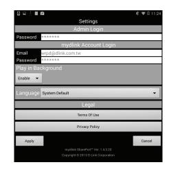
6. You can now use the mydlink SharePort app interface to stream media and access files stored on your removable drive. The wireless icon at the bottom will be lit green to indicate you are connected to the router through Remote Access.
