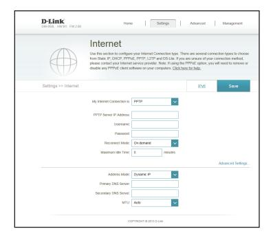
**Secondary DNS** Enter the secondary DNS server IP address assigned by your ISP. **Server**:
