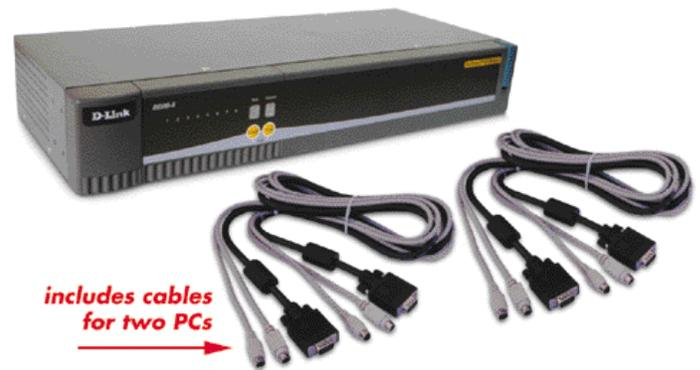
*D-Link's DKVM-8 controls 8 different Server PC's w/ 1 keyboard and incorporates a User-Friendly Interface*
