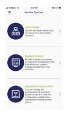
The next step is to select an AP provision profile. The profile is used to push to the selected DAPs. Tap **Quick Setup** to begin the deployment of a standalone DAP to the Nuclias Connect server.
