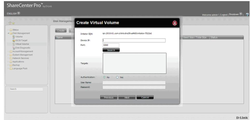
Under **Device IP**, enter the IP address of the **iSCSI Target**. This can either be an **IPv4** or **IPv6** address. Click the **Search** button
