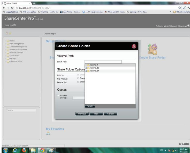
Under Volume Path, select the path by clicking once on the open field. A drop down menu appears of the drives on your NAS.
