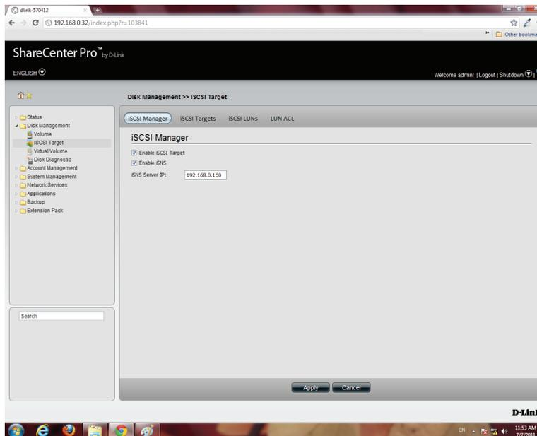
Click the Enable iSCSI Target checkbox to enable this function.
