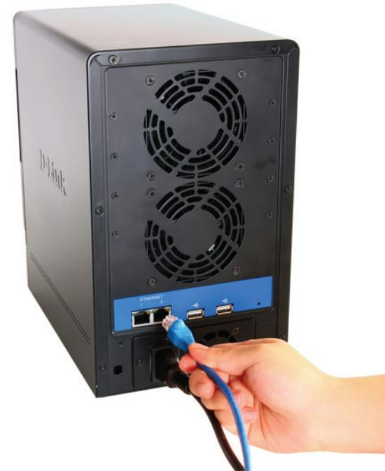
6. Connect the supplied power adapter to the power receptacle.
