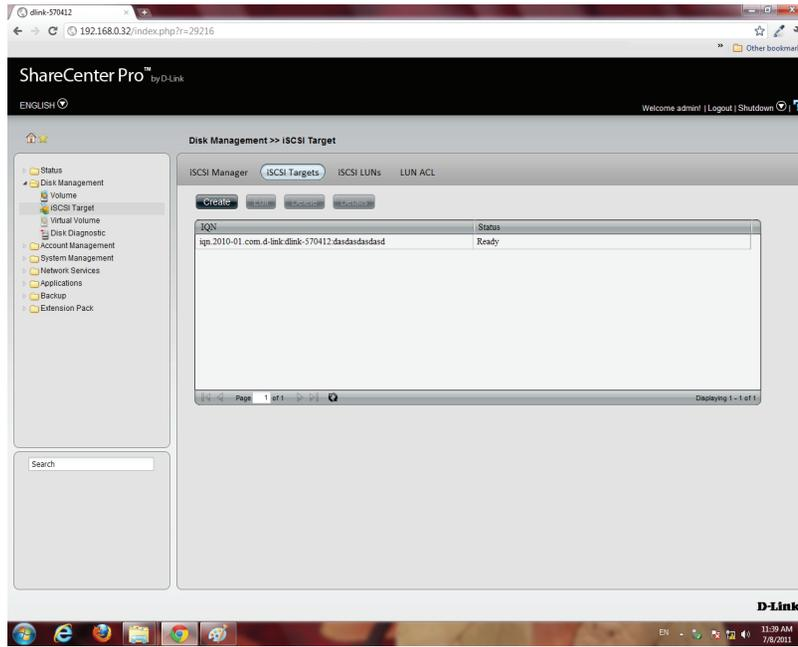
The newly created iSCSI Target appears in the iSCSI Target table.
