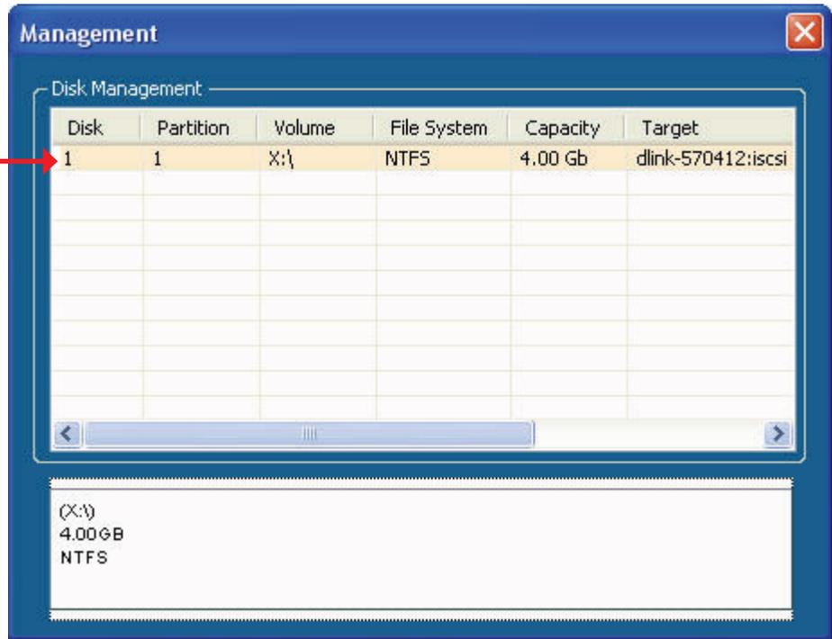
3. The newly mounted disk is displayed in the My Computer window and can be used as if it was a locally attached disk.
