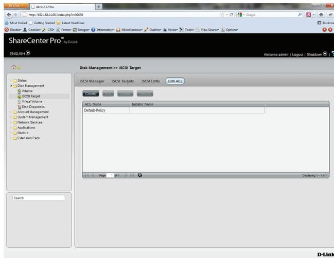
The Default Policy will always be first ACL on the LUN ACL table when the iSCSI Target service is enabled.
