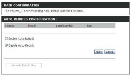
Monitoring: To monitor the progress of the Auto Rebuilding process, you can go to STATUS > SYSTEM INFO and monitor the Sync Time Remaining (progress of the Rebuilding process).
