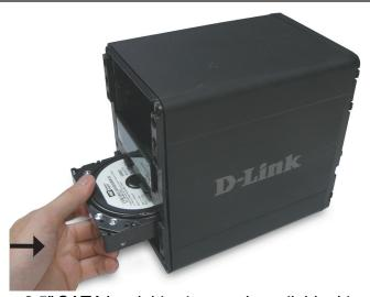
3. Insert a 3.5" SATA hard drive into each available drive bay. Make sure to align the drive connectors to the SATA connectors on the bottom edge inside the drive bay of the DNS-343. Gently push the drive in until it connects. When a drive is inserted properly, you will feel it "seat" into the connector. Some hard drives that are thin or oddly shaped may need to be guided carefully into position.
