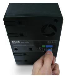
5. Connect an Ethernet cable to the available Ethernet port. This cable should connect the DNS-343 to your local network via a router or switch, or directly to a computer for configuration.
