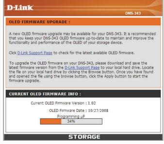
▲ To complete the OLED firmware upgrade process, please disconnect the power cord from the NAS.
