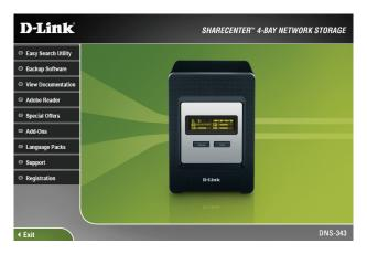
Click Easy Search Utility. The Easy Search Utility will load and detect any DNS-343 devices that are on the local network. If the DNS-343 you are working with does not show up in the device list, click Refresh.
