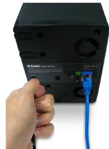
6. Connect the supplied power adapter to the power receptacle.7. Connect a USB printer. (Optional)
