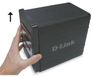
1. Access the drive bays by sliding the faceplate up until it unlatches from the device.
