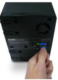
5. Connect an Ethernet cable to the available Ethernet port. This cable should connect the DNS-343 to your local network via a router or switch, or directly to a computer for configuration.
