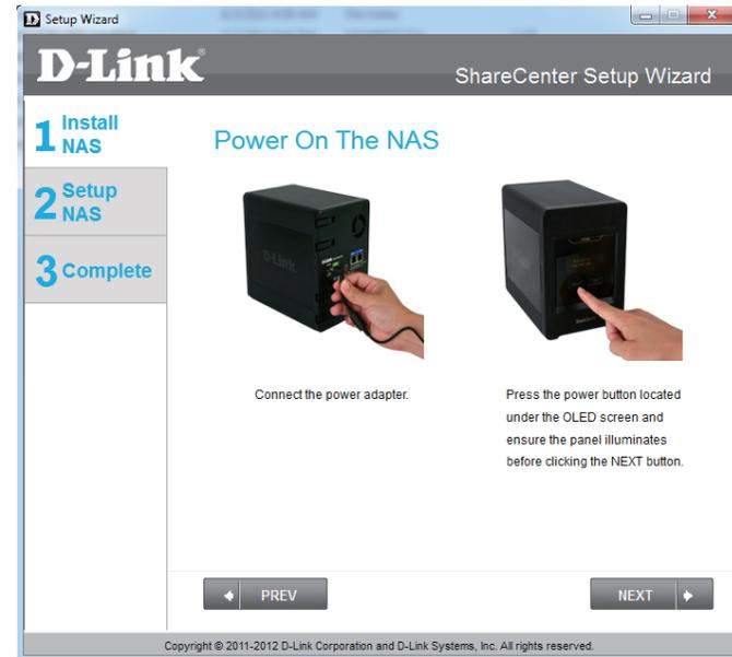
**Step 8** - With the power on, press the **Next** button on the device and check and make sure the IP address of your ShareCenter matches what you see on the screen.
