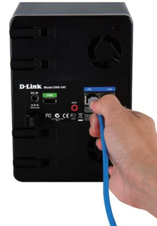
**Step 4** - Connect an Ethernet cable to the LAN 1 Ethernet port. This cable should connect the ShareCenter to your local network via a router, switch, or directly to a computer for configuration.
