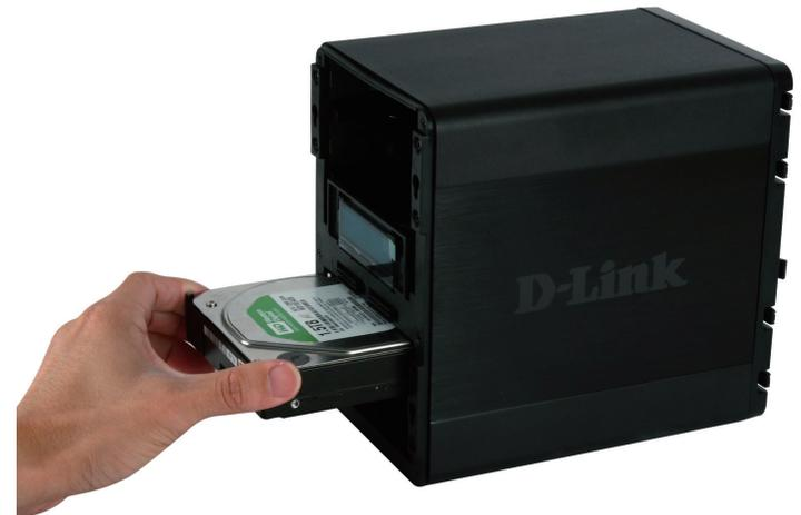
**Step 2** - Insert up to four 3.5" SATA hard drives into the drive bays.
