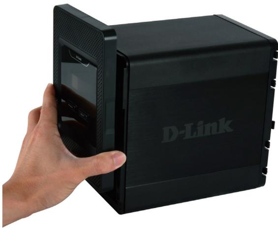
**Step 1** - Remove the front panel by firmly gripping the panel and sliding it up until it unhooks. Then remove it to allow access to the drive bays.
