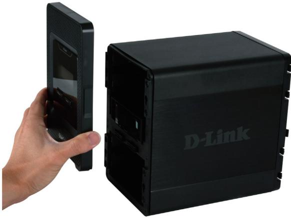
**Step 3** - Re-attach the front panel. Align the 4 panel hooks with the corresponding slots on the chassis and slide the front panel down until it is firmly seated.
