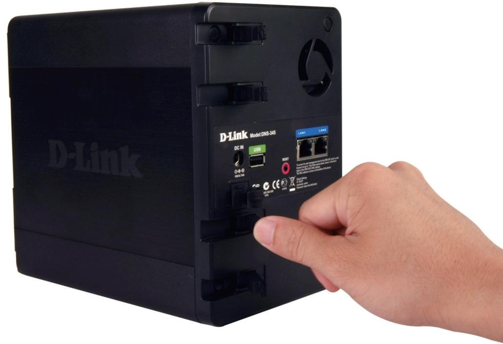
Pull the rear levers to disconnect the hard drive(s) from the SATA sockets.
