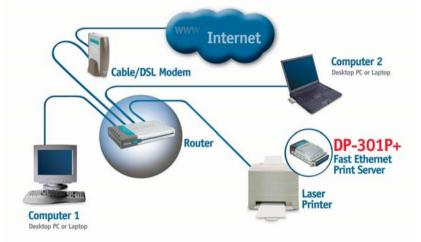
Next, make sure that the Printer is turned **OFF**. Connect the parallel end of the DP-301P+ to the parallel port of the printer
