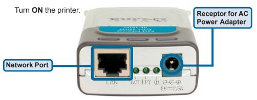
Then, plug one end of the power adapter into the DP-301P+ and the other end into your electric outlet. The DP-301P+ will turn on and begin a self-test.
