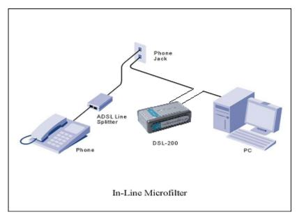
**Note:** Do not install the microfilter between the Modem and the telephone jack. Microfilters are only intended for use with regular telephones, Fax machines and other regular telephone devices.
