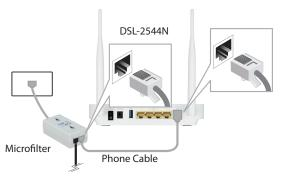
Connect the Ethernet cable from Ethernet port on your computer. Connect the Ethernet cable from the LAN port of the modem router to the
