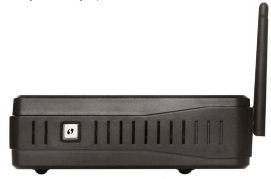
The WPS Push Button is located at the right side of the Router. Press the button to enable the WPS function. The light blinks when WPS is successfully triggered. When the connection is successfully established between the Router and the client, the blue light will be solid and remain for five seconds. After the light is off, the Router is ready for configuring a new WPS connection.
