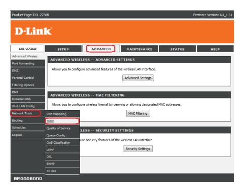
9. Tick [Enable IGMP Snooping] box under IGMP SETUP page
