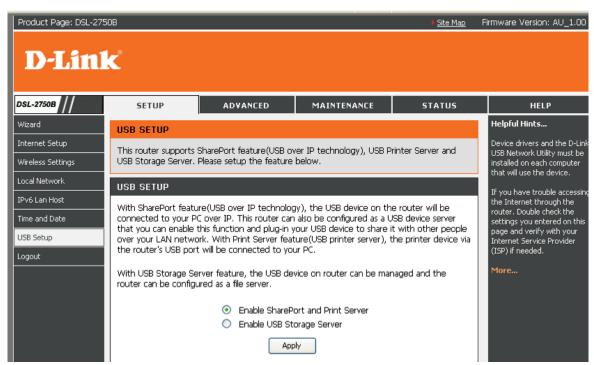
To setup Printer Server, press **setup** button in **USB SETUP** window enter the server configuration page
