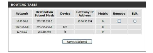
The routing information protocol (RIP) is one of the most commonly used interior gateway protocol (IGP) routing protocols on internal networks (and to a lesser extent, networks connected to the Internet), which helps routers dynamically adapt to changes of network connections by communicating information about which networks each router can reach and how far away those networks are.
