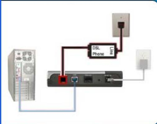
Connect the microfilter/splitter (optional on some models) to the **telephone jack**. Connect the device's Line port to the microfilter/splitter **DSL jack**.
