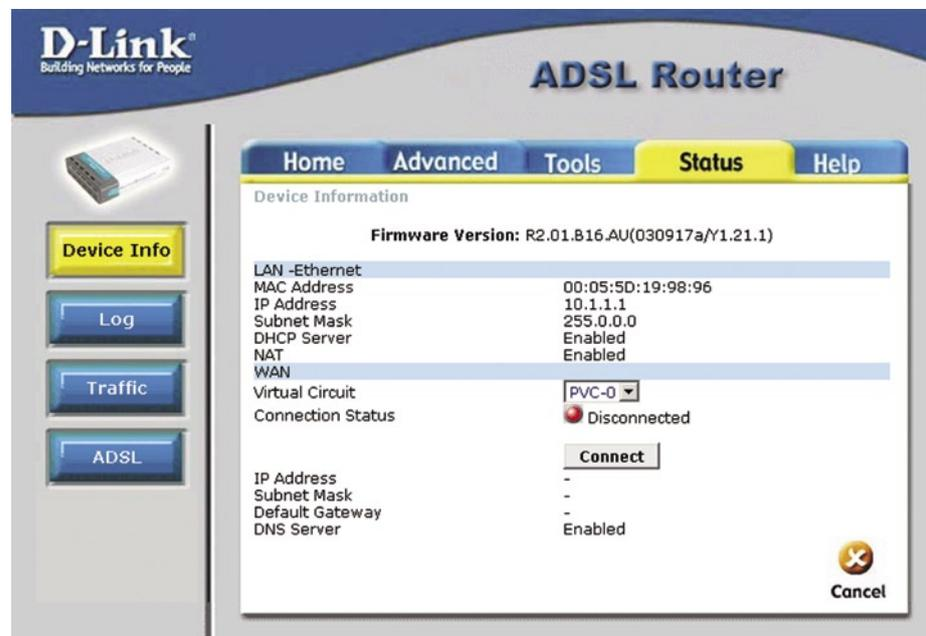
Configuration Utility makes it easy to quickly set up and configure the DSL-504G. It displays a wide array of management settings and tools.
