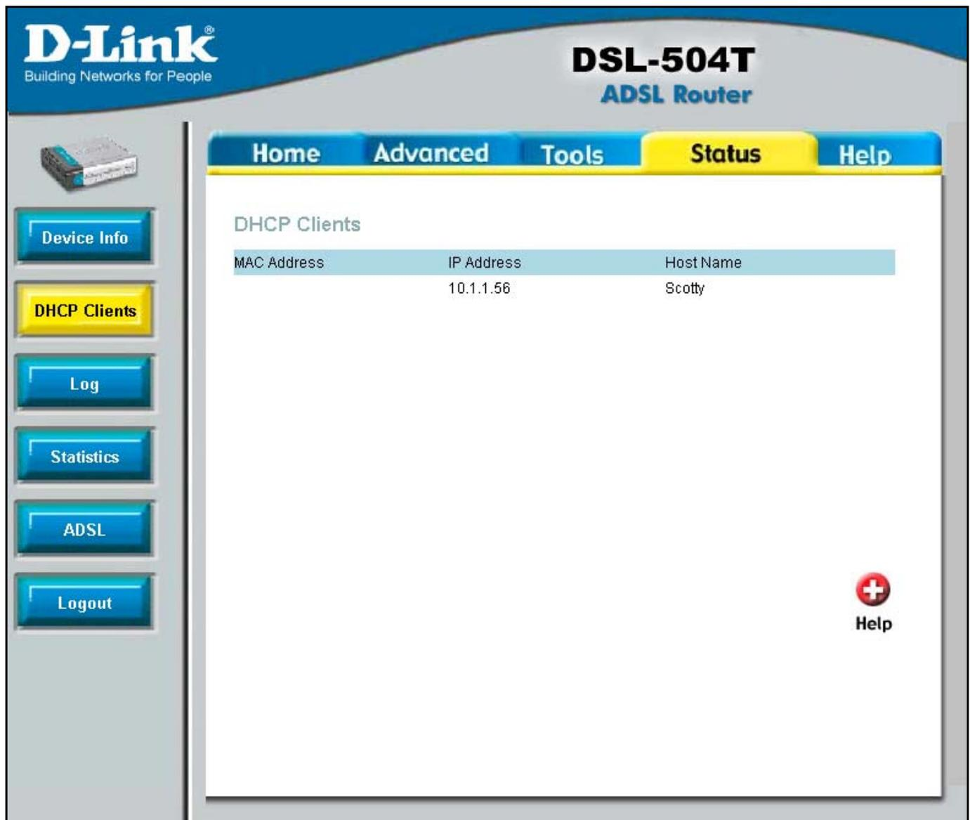
The screenshot shows the web interface of a D-Link DSL-504T ADSL Router. The top navigation bar includes 'Home', 'Advanced', 'Tools', 'Status' (highlighted), and 'Help'. The left sidebar contains buttons for 'Device Info', 'DHCP Clients' (highlighted), 'Log', 'Statistics', 'ADSL', and 'Logout'. The main content area displays the 'DHCP Clients' page with a table listing connected clients.
