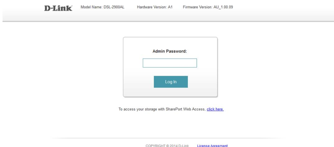
*If you cannot recall the password you assigned to your modem you will need to reset the modem to factory defaults by pressing the reset button for 10 seconds. Please note that this will revert all the settings in the modem to factory settings and you will have to reconfigure it with your Internet settings and Wireless security. Make sure you have your Internet account details (given by your Internet Provider) handy.*
