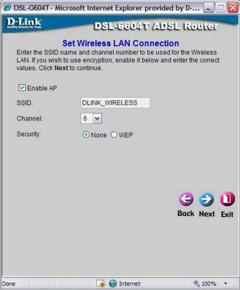
The screenshot shows a web browser window titled "DSL-G604T - Microsoft Internet Explorer provided by D-...". The page header includes the D-Link logo and "DSL-G604T ADSL Router". The main heading is "Set Wireless LAN Connection". Below this, there is a text box with instructions: "Enter the SSID name and channel number to be used for the Wireless LAN. If you wish to use encryption, enable it below and enter the correct values. Click **Next** to continue."
