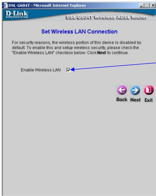
Check this box to enable wireless access to the Router.
