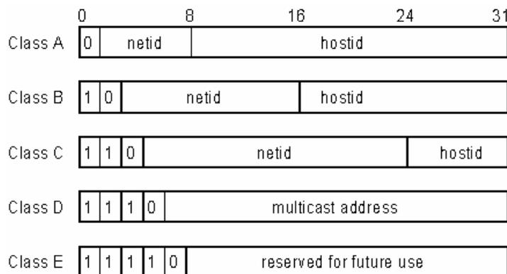
Networks attached to the Internet are assigned class types that determine the maximum number of possible hosts per network. The previous figure illustrates how the net and host portions of the IP address differ among the
