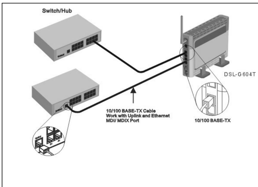
If you wish to reserve the uplink port on the switch or hub for another device, connect to any of the other MDI-X ports (1x, 2x, etc.) with a crossed cable.
