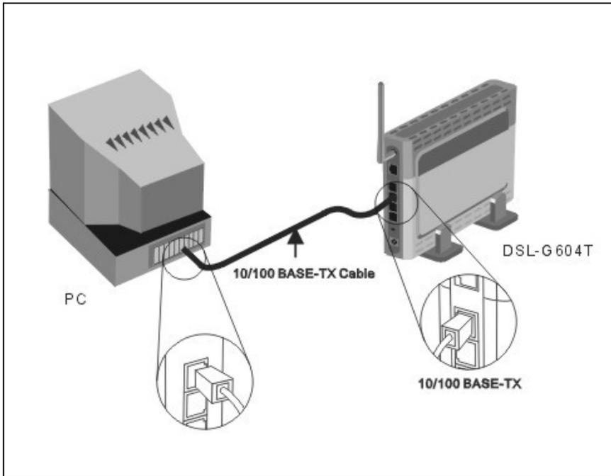
You can connect the Router directly to a 10/100BASE-TX Ethernet adapter card (NIC) installed on a PC using the Ethernet cable provided as shown in this diagram.
