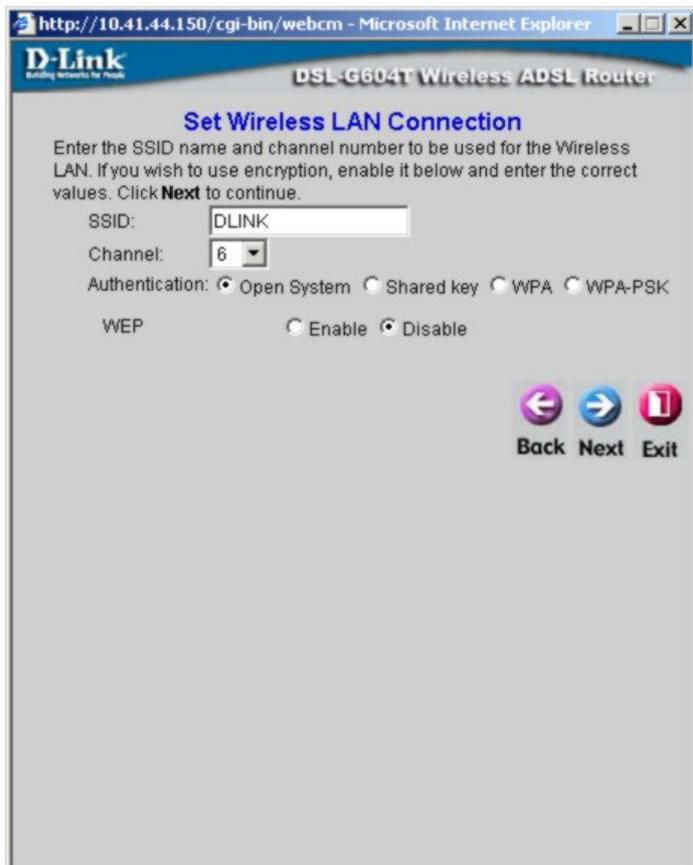
Configure the **SSID** and **Channel** according to the requirements of your network. The default settings use an **Open System** for wireless **Authentication** and WEP is disabled. Open System Authentication to allow any wireless station to associate with the access point. You can accept the default settings and click **Next** to proceed to the final step. Wireless LAN security can be configured at any time using the Wireless menu in the Home directory.
