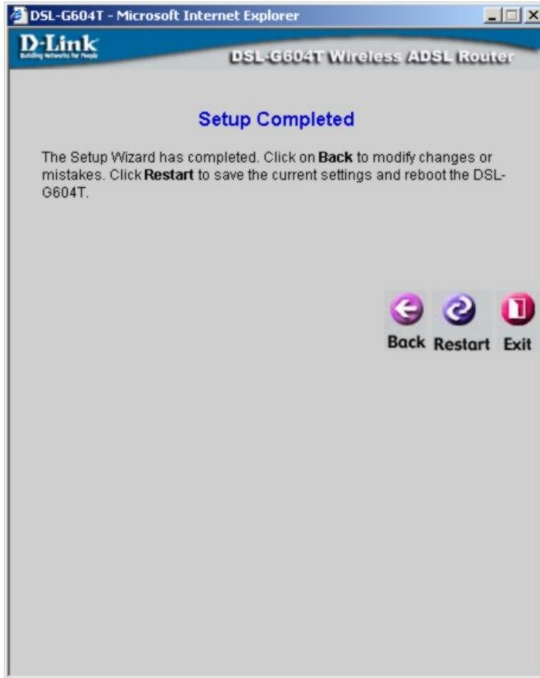
Do not turn the Router off while it is restarting. When it is finished rebooting, click **Close** to close the box and continue to configure the Router as desired.
