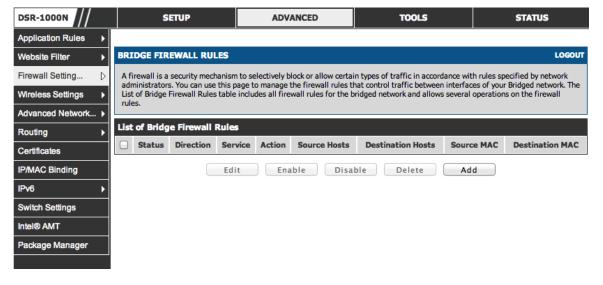
Firewall rules configured for the bridge will filter traffic based on protocol, outgoing range of ports and/or the incoming range of ports. The processing is at L2 and can apply either to the LAN1 port or the WAN2/DMZ port (not both).
