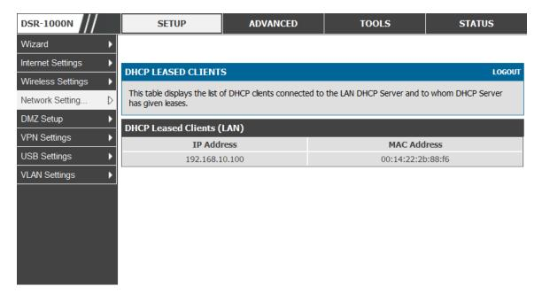
**IP** Addresses: The LAN IP address of a host that matches the reserved IP list. **MAC** Addresses: The MAC address of a LAN host that has a configured IP address reservation.
